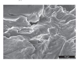
The SEM is used as well for the characterisation of structures. We show here an etched ceramographic section as an example. The light microscope cannot expose the extremely fine-grained structure of a dispersion ceramic of aluminium oxide and zirconium oxide in the sub micrometer range.
