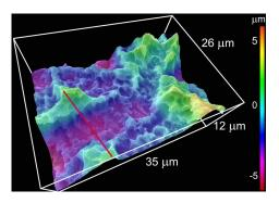
We defined a cross-sectional profile along the red line in the above image and depicted it below after filtering of the waviness. The thus established roughness values are  $R_{\alpha} = 140 \text{ nm}$  and  $R_{z} = 446 \text{ nm}$ .
