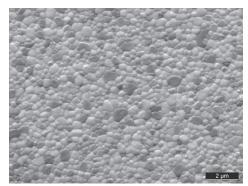
The following image comes from an examination of a drill bit with a hard wear protection coating (thin layer). The slightly porous layer shows many fissures in the proximity of the breaking edge. Yet, the fact that there are hardly any layer chips indicates a good coating adhesion.
