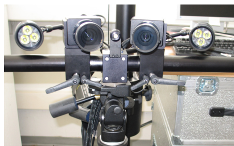
Figure 2: Camera system for optical deformation measurement (gom ARAMIS/PONTOS 2M).
