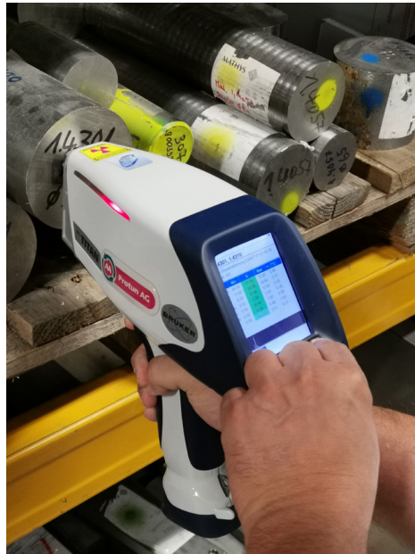
Figure 2: Mobile handheld X-ray fluorescence spectrometer (ED-XRF measuring method).
