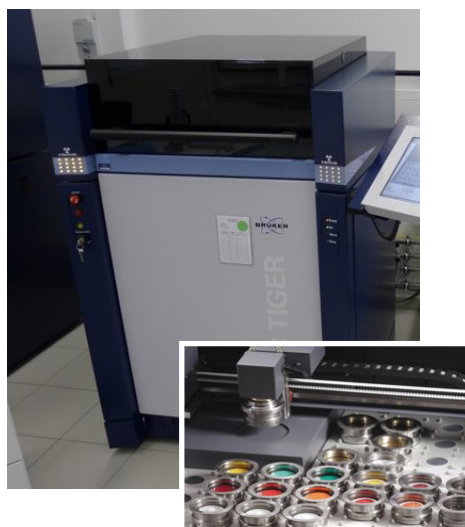
Figure 3: Stationary X-ray fluorescence spectrometer (WD-XRF measuring method).
