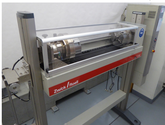
Figure 1: Zwick's TL500 torsion testing machine, with extension for simultaneous static tensile- or compression loading.
