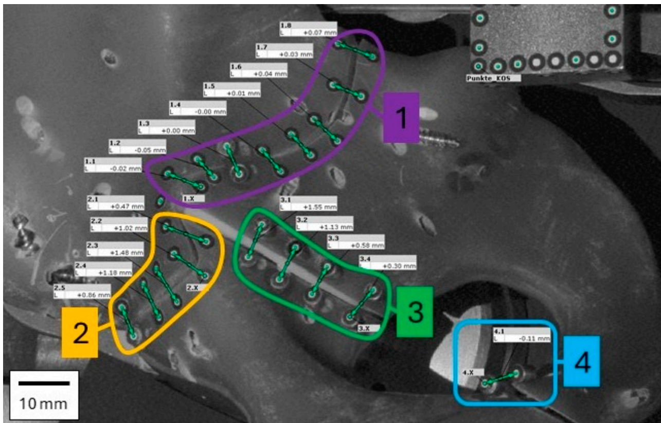
Figure 4. Detailed view of the software evaluation of the relative point distances (corresponds to prior photograph in Figure 1). These represent a 2D visualization of a 3D point cloud. The points at the top right are used to determine a constant coordinate system (not shown in other figures). The four mentioned zones are marked for clarity (compare with Figures 1 and 5).
