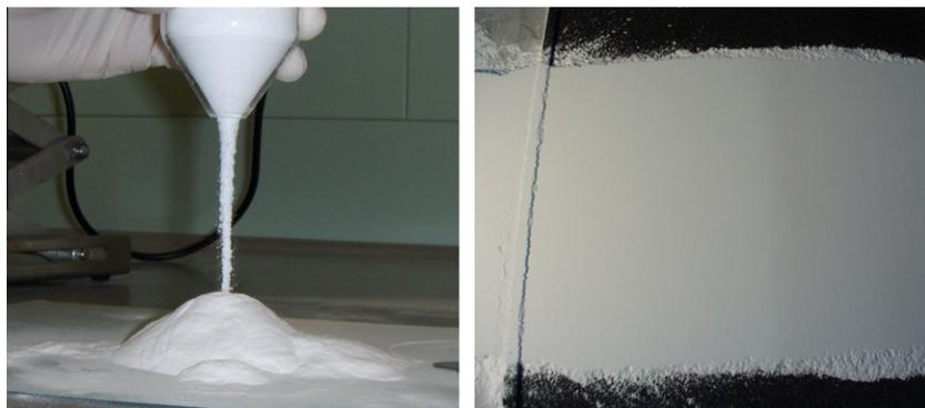
Fig. 8. High flowability of plasma treated 5  $\mu\text{m}$  powder (left) and a homogeneous bed of the same powder (right).
