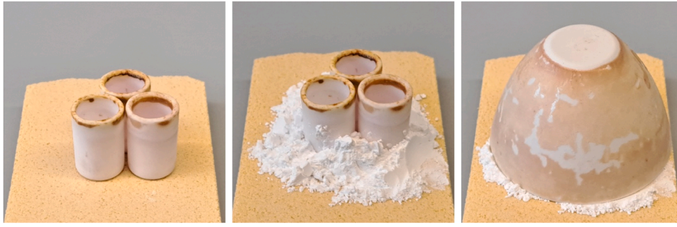
Fig. 1. Experimental setup for the calcinations. Left: Samples calcined in open atmosphere. Center: Sacrificial monetite was placed around the samples. Right: The samples and sacrificial monetite were covered with another crucible to minimize the gas volume over the samples during the calcination in saturated atmosphere.
