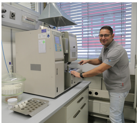
Figure 1: CGHE analyser (LECO CS 230) for carbon and sulfur analyses
