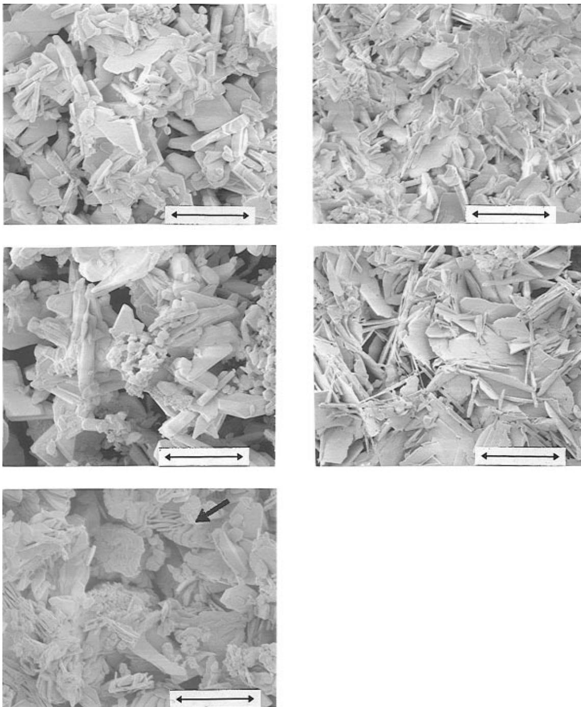
**Figure 3**—Initial microstructure of cements made of 1.3 g of  $\beta$ -TCP, 0.7 g of MCPM, and (a, top left) 1.6 mL of deionized water and 20 mg of GS; (b, top right) 1.6 mL of deionized water and 100 mg of GS; (c, middle left) 2.4 mL of deionized water and 20 mg of GS; (d, middle right) 1.92 mL of deionized water, 0.4 g of CSH, and 20 mg of GS; (e, bottom right) cement shown in c after release. The bars correspond to 10  $\mu$ m. The arrow on Figure 3e shows a layered crystal.
