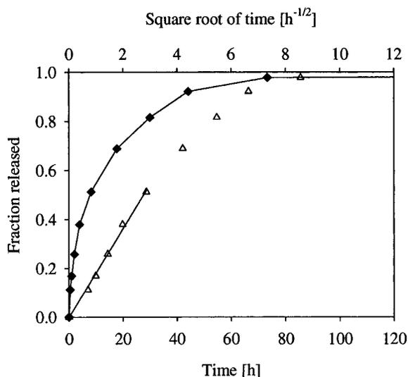
**Figure 5**—Linearization of a GS release curve. The GS fraction released is plotted as a function of (♦) time or ( $\Delta$ ) square root of time. The slope of the linear domain is  $k = 0.182 \text{ h}^{-1/2}$ .
