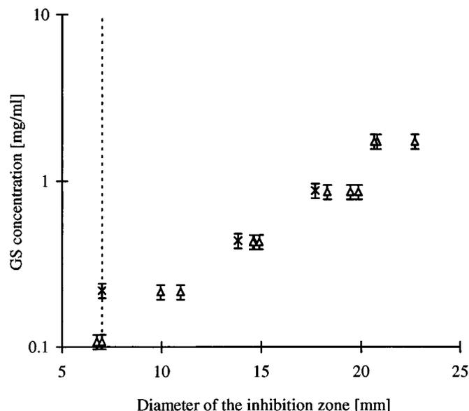
**Figure 9**—Biological activity of GS ( $\times$ ) before and ( $\triangle$ ) after mixing with the cement. The size of the error bars corresponds to  $\pm 1.96$  standard errors. The dotted line corresponds to the bore hole diameter.
