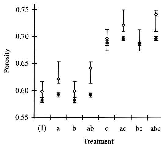
**Figure 7**—Comparison between the initial and final porosity of the cement samples used in the multifactorial experimental design  $2^3$ . Factor A: amount of CSH; Factor B: amount of GS; Factor C: amount of mixing liquid. Key: (♦) initial porosity; (◇) final porosity. The size of the error bars corresponds to the 95% confidence interval of and around the adjusted values (not shown on the chart for clarity reasons).
