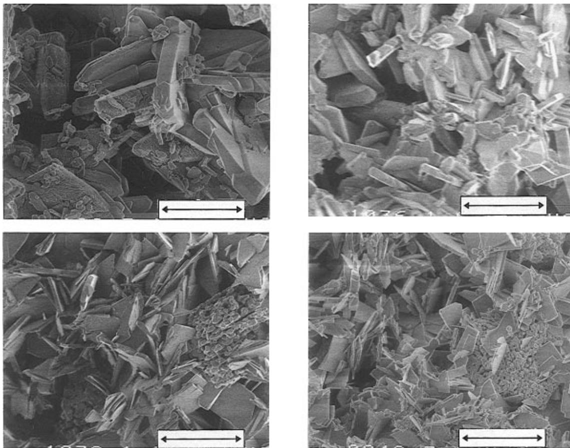
**Figure 2**—GS effect on the initial microstructure of cements made of 1.2 g of  $\beta$ -TCP, 0.8 g of MCPM, 2 mL of deionized water: (a, top left) 0% GS; (b, top right) 3% GS; (c, bottom left) 9% GS; (d, bottom right) 16% GS. The bars correspond to 10  $\mu$ m.
