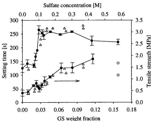
**Figure 4**—Effect of the amount of GS on the setting time (upper curve) and the tensile strength (lower curve) of the cement. Composition: 1.2 g of  $\beta$ -TCP, 0.8 g of MCPM, 2 mL of solution. Key: (●) GS dissolved in solution, average value ( $n = 3$ ); ( $\Delta$ ) GS added as powder, data points; (○): GS dissolved in solution, data points (only for tensile strength). The error on the mean is given at a 95% confidence level.
