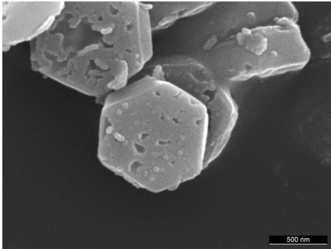
Fig. 3.  $\beta$ -Tricalcium phosphate plates obtained according to the method of Tao et al.<sup>100</sup>
