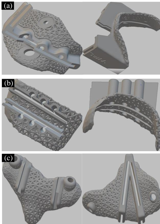
Fig.2. 3D model of different types of HTO jigs: (a) Open wedge surgical jig; (b) Closed wedge surgical jig; (c) Complex surgical jigs.
