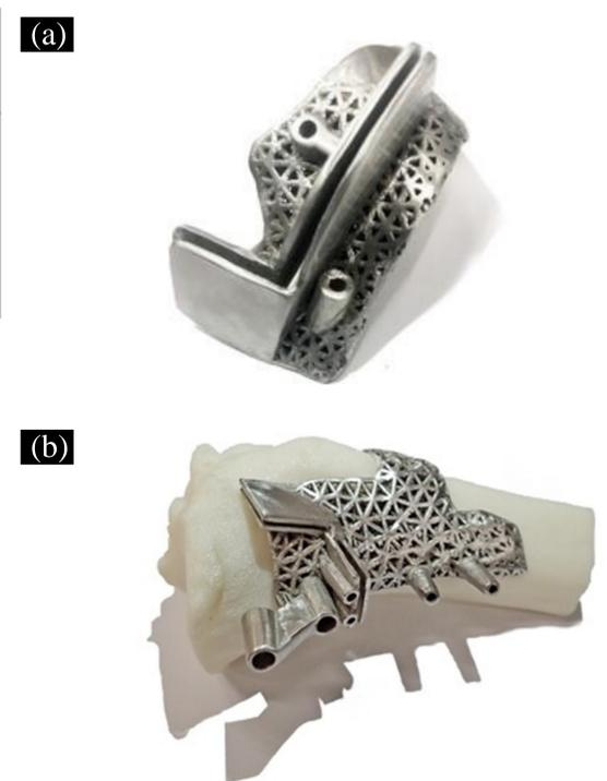
Fig.3. Finished HTO surgical jig product after post-processing (a) shows customized cutting guides and k-wire guides. 3D anatomical model could be used to verify the surface compliance of 3D-printed HTO surgical jigs with patient anatomy (b).
