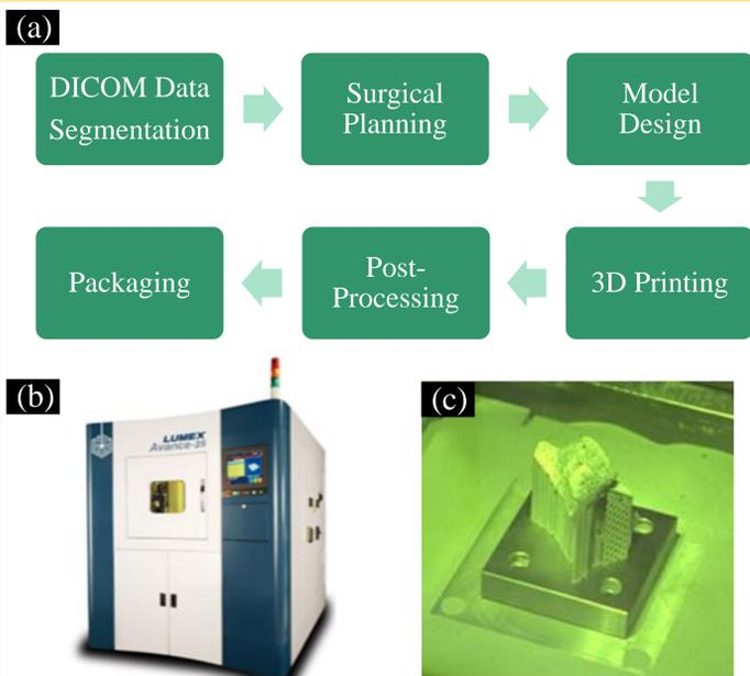
Fig.1. Design and manufacture of HTO surgical jigs: (a) Workflow of the production of patient-specific surgical jigs by additive manufacturing; (b) The Matsuura LUMEX Avance-25 printer used in manufacture process; (c) 3D-printed jig before post-processing.
