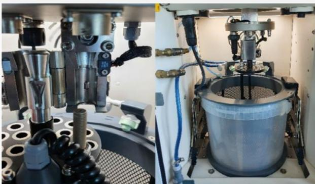
Fig. 2: Holder for the graphite clamping rods (left). Samples inserted in the polymeric electrolyte (right).
