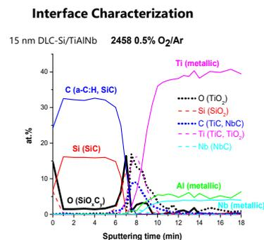
Fig. 4: XPS depth profile separated into components
