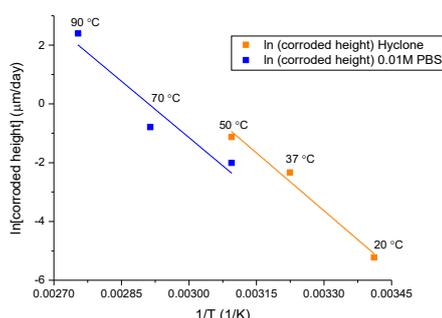
Fig. 3: Arrhenius plot demonstrates linear relationship of the Si uniform corrosion rate with temperature in confined space, when immersed in 0.01 M PBS and HyClone Wear Testing Fluid
