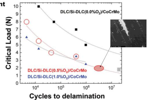
Fig. 6: Wöhler-like curve of the interface failure. Insert shows failure in a simulator.
