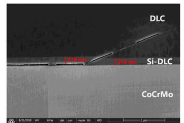
Fig. 7: FIB cut near the interface: plastic deformations and delaminated areas are visible
