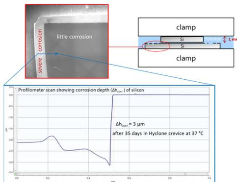
Fig. 2: Crevice/confined space experimental setup: Profilometer scan shows significant corrosion depth of 3 μm in the confined space outside of a Si crevice, after 35 days immersion in HyClone® Wear Testing Fluid at 37 °C
