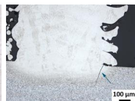
Etched cross-section with hardness indents (left) and detailed view with a secondary crack at the interface (right)
