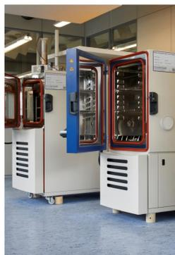
Figure 2: View of the two chamber oven where the DUT are going through accelerated ageing 0 - 150°C
