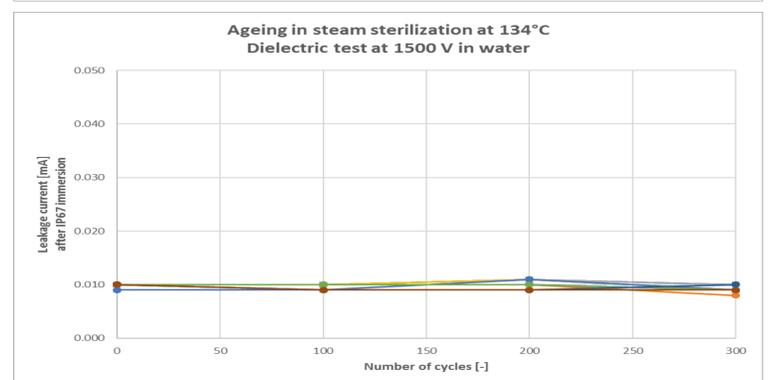
Figure 4: Leakage current measurement after different ageing processes
