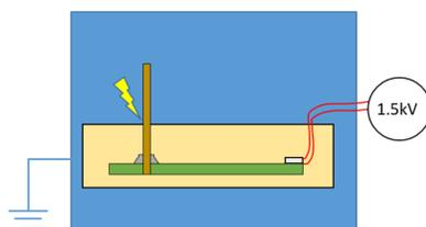
Figure 3: Scheme of the dielectric test and potential ingress point inducing current leakage
