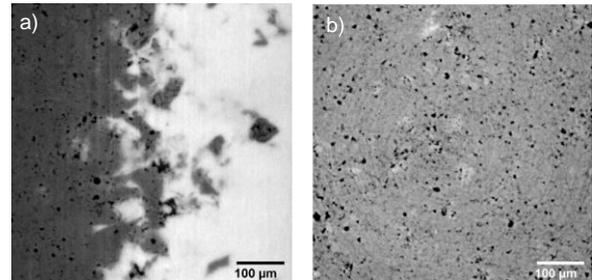
Fig. 3: a) Reconstructed SXR $\mu$ CT images of the substrate- $\text{Al}_2\text{O}_3$  coating interface. b) Reconstructed cross-section through the  $\text{Al}_2\text{O}_3$  coating.
