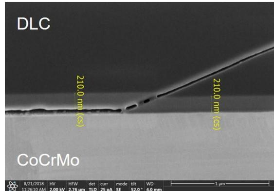
Fig. 2: FIB cross section of a growing crack in 4 µm DLC/Si-DLC (1.0 % O<sub>2</sub> contamination)/CoCrMo after 13500 cycles in PBS. Plastic deformations of the Si-DLC are visible [3].
