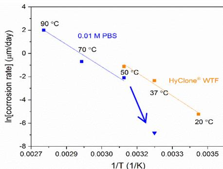
Fig.1: Arrhenius plot of Si in a crevice/confined space arrangement. Corrosion rate measured in the confined area at different temperatures, from [2].
