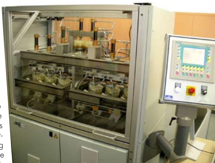
Figure 1: Servohydraulic 6-stations hip and spine simulator.
